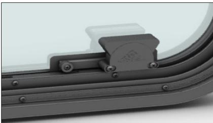
**ROCKER LATCH:** The rocker latch provides the greatest visibility and control to the driver. The rocker latch allows the driver to effortlessly open and secure the window in various positions; the strikes can be set to open at various increments of 2.75".
