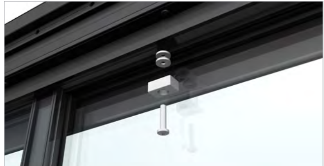
Figure 1 - Removal of Philips head screw, sash stop & two (2) washers from transom insert.
