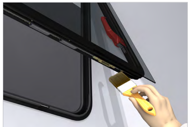
Figure 2 - Removal of build-up on emergency release bar.
