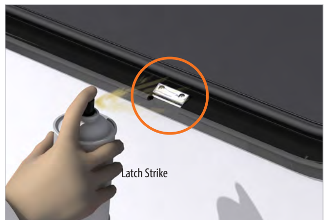
Figure 3 - Application of dry film lubricant to latch strikes.
