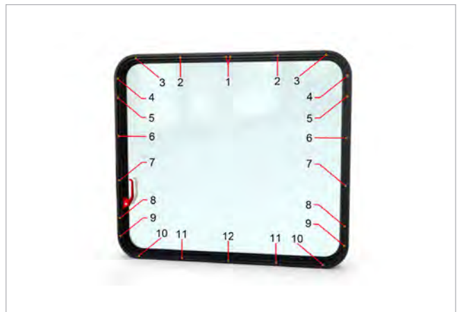
Figure 5 - Sequence for tightening clamping screws.
