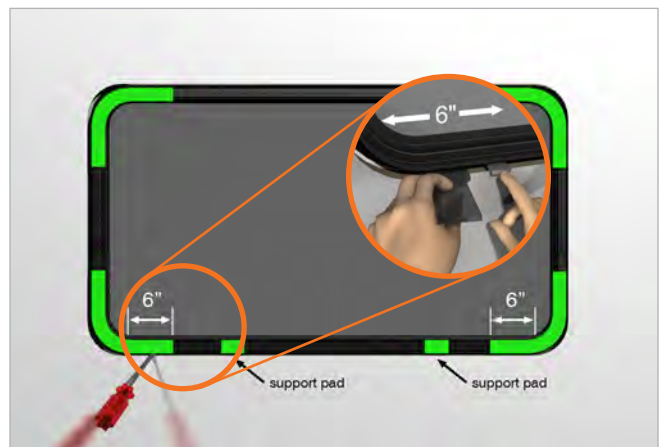
Figure 3 - Adding shims under window support pads.
