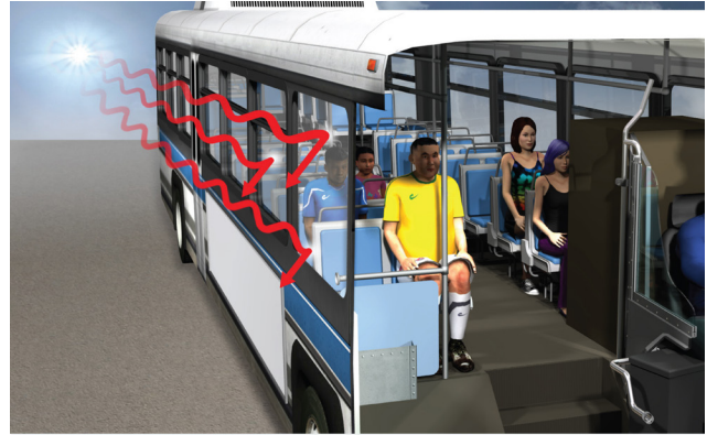
With the use of Solar Management Glazing the overall operator and passenger comfort is improved as the net influence of solar energy transmittance is reduced.
