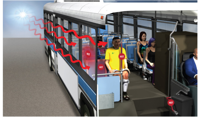
Without the use of Solar Management Glazing the heat from the sun penetrates the bus having a negative effect on passenger comfort.
