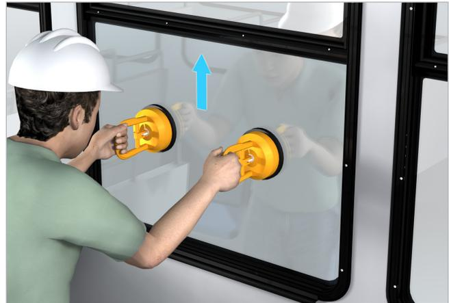
Figure 1 - Placement of suction cups.
