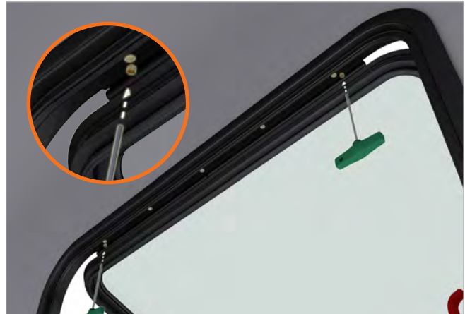
Figure 1 - Removal of retaining screws under transom.
