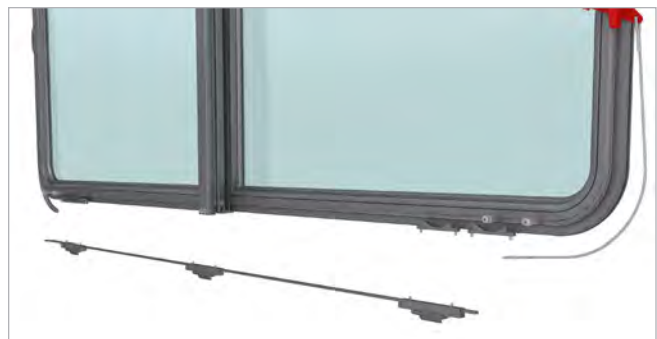
Figure 3 – Removal of emergency release bar.
