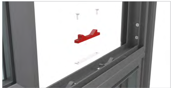
Figure 2 - Removal of broken strike.
