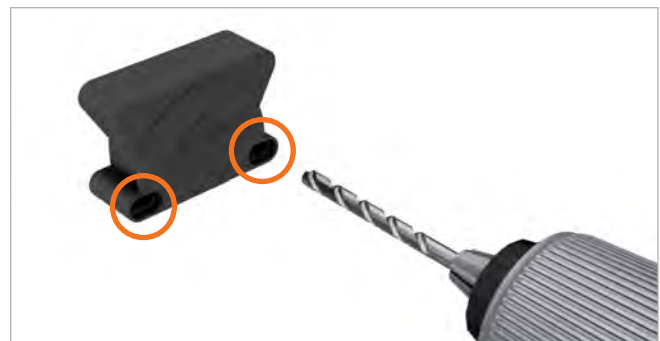
Figure 3 – Drilling two (2) slots through rocker latch.
