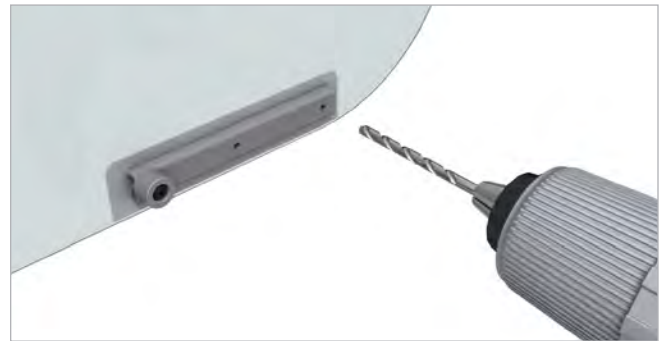
Figure 2 – Drilling through aluminum latch mounting base.
