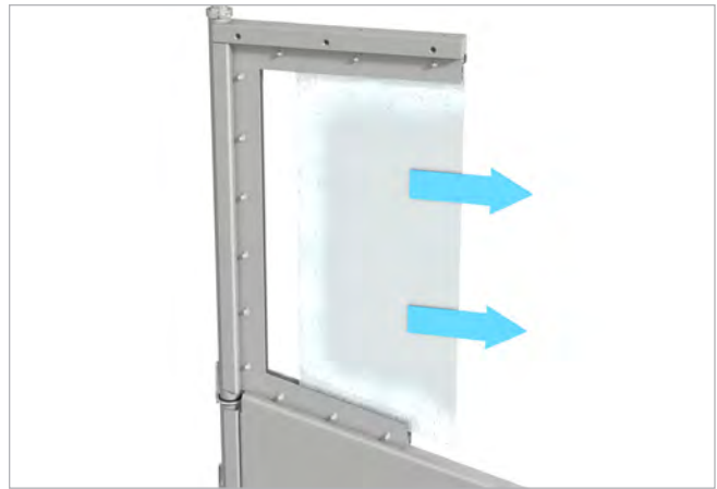
Figure 4 – Removal/replacement of fixed glass.
